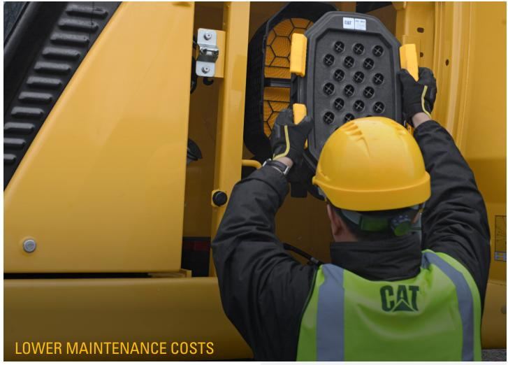
With extended maintenance intervals, you get more done at a lower cost compared to the 336F. Consolidated filter locations make service faster. Hydraulic, air, and fuel tank filters have increased capacity and longer life.
